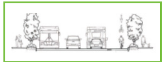
Transit-Only EmX Contraflow Lane, 67 feet
